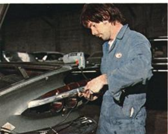
Work in progress: This is Garner making headlights out of tail-lights. Clips hold the lenses up so the Chevy can drive at night.
